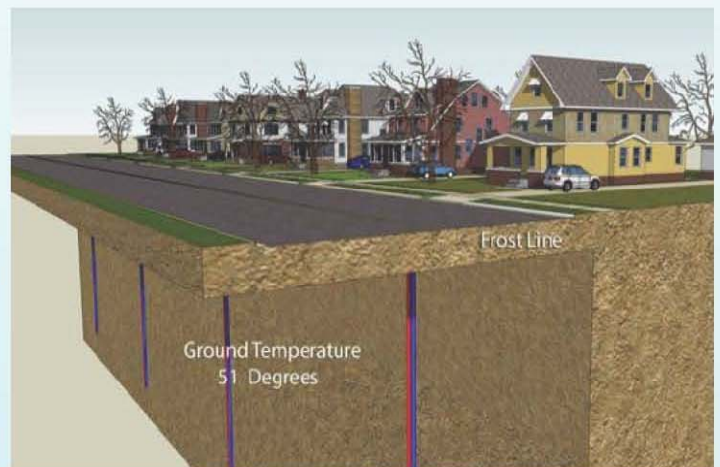
Diagram of a Residential Geothermal Energy System – Vertical blue and red lines depict the heat exchange well that services the Ground Source Heat Pump (GSHP) located in the home. Optional function – GSHP waste heat can preheat an electric water heater.
