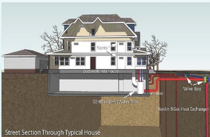
Diagram of a Residential Geothermal Energy System – Vertical blue and red lines depict the heat exchange well that services the Ground Source Heat Pump (GSHP) located in the home. Optional function – GSHP waste heat can preheat an electric water heater.
